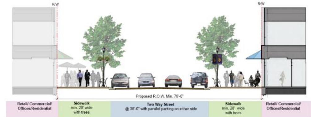
Typical Local Street Cross-section
